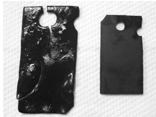
ASTM D 471 Volume Swell sample after aging 480 hours @ 250° F . (Samples shown 3/4 size)
