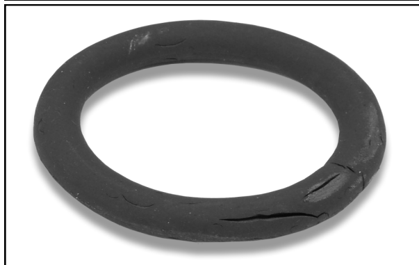
Example of a damaged O-Ring made from FKM that was not RGD Resistant.
